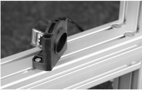
Before starting to mount the muting sensors, check the section for the mounting position with respect to the muting type. Mount the muting sensor according to its instruction.
