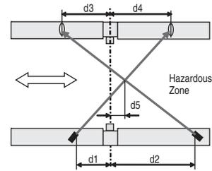
Figure 20: The distance  $d5$  should be as short as practicable in order to avoid persons entering the hazardous zone without being detected when following immediately after the pallet or the transport system. The muting beam cross point has to be in the hazardous zone.
