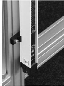
Use the integrated laser alignment system (ILAS) for easy verification. Touching the symbol
