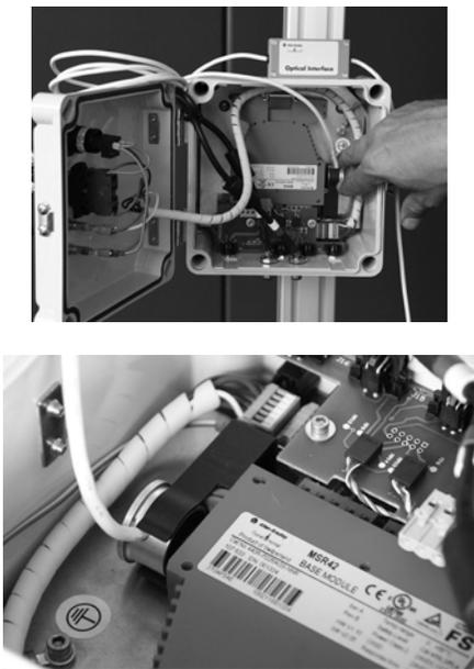
In case the default configuration (see above) will not be used, the created configuration has to be downloaded with the optical interface (445L-AF6150); connected to the MSR42 control module.
