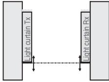
Position the emitter and receiver light curtain at the same height on the mounting column.
