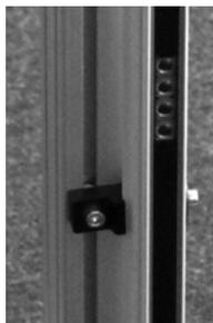
The GuardShield Micro 400 reinforced profile uses the same mounting brackets (445L-AF6140) as the GuardShield Safe 4. They are supplied with the light curtain.
