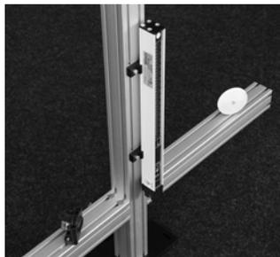
**Note:** The image shows the RightSight with reflector. Normally, the muting sensor gets mounted on one mounting bar and the reflectors on the other side.
